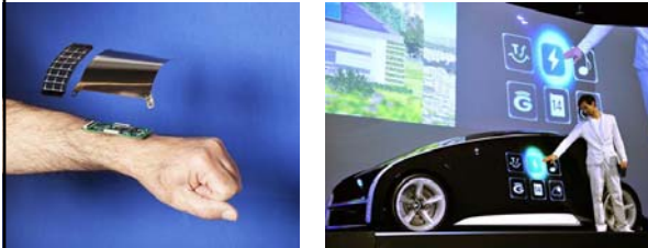
Components of the wrist-worn display prototype developed at HP Labs are shown in this illustration. When completed, the device will incorporate a working flexible display powered by solar cells.
