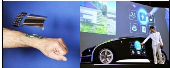
Components of the wrist-worn display prototype developed at HP Labs are shown in this illustration. When completed, the device will incorporate a working flexible display powered by solar cells.
